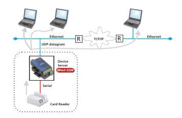
As an example, consider the situation illustrated in the above figure. In this case, the application dictates that card reader data should be sent to more than one host, all of which are connected to the Internet. The way to enforce such a requirement is to configure the device server connected to the card reader for UDP Server/Client mode, and then set up the system so that data are sent to each of the hosts.
