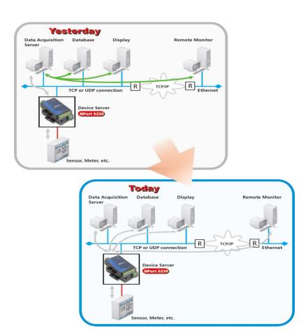
For example, as illustrated in the figure shown here, a 2-port serial device server shares its ports with 4 different hosts.
