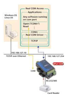
The figure shown here nicely illustrates a typical scenario of a device server configured for Single-Host application. In this case, a Card Reader is attached to a device server with IP address 192.168.127.254. The device server's Ethernet port is attached to a LAN, generally by using a straight-through Ethernet cable to connect to a hub or switch. A host computer with IP address set to 192.168.127.10 is connected to the same LAN.
